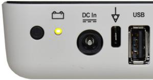
The unit can either be operated from the mains supply or from the built-in rechargeable battery. Battery charging is indicated by the LED below the battery symbol.
