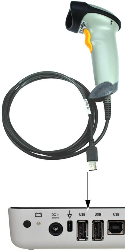
A barcode reader can be attached to the USB port on the back panel to read the Patient ID / Visit ID. SCHILLER has tested the following barcode reader:
