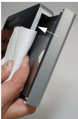
Over a period of time, the printing ink from the grid on the paper can form a film on the thermal print head. This can cause the print quality to deteriorate. We recommend therefore that the print head is cleaned with alcohol every month. This is done as follows:
