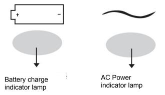
When AC power is turned off and system power is turned on, the equipmen is operated from battery power. When battery power in on, battery charge indicator lamp is illuminated green. When battery power is low, buzzor alarms three times in series and battery charge indicator lamp is illuminated yellow. In this case, turn the system power off and connect the AC power source. Then turn the system power on again.
